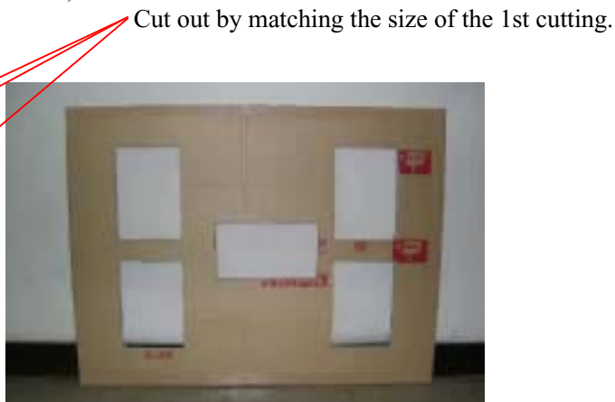
(Fig. 4 - As for the 2nd flattened cardboard box, cut out the shape in the same way as Fig.2. All cardboards are cut out as below.)
