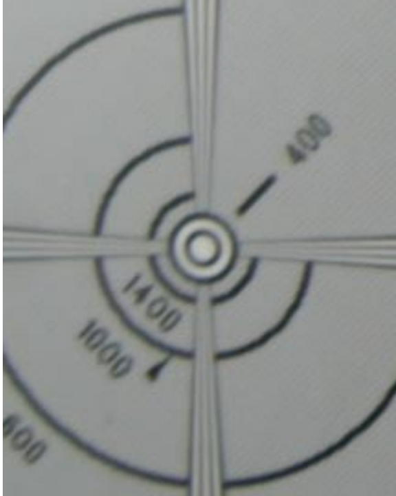
Defective at WIDE side
