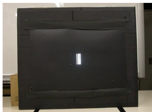
(Fig. 6- Setting board is blackened with the chart being attached.)
