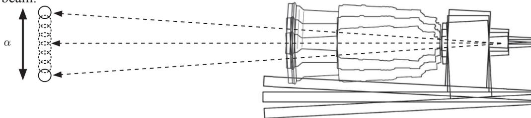
**Notes:** During the above measurement, laser spot light swings from side to side and up and down. This phenomenon is caused by operations of the VR unit control so NOT defective.
