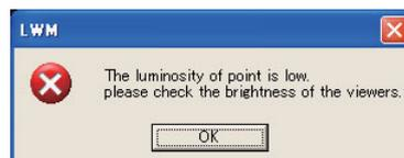
**Note 2: When the below warning is given, recheck that the Quality mode of the camera is set to RAW.**
