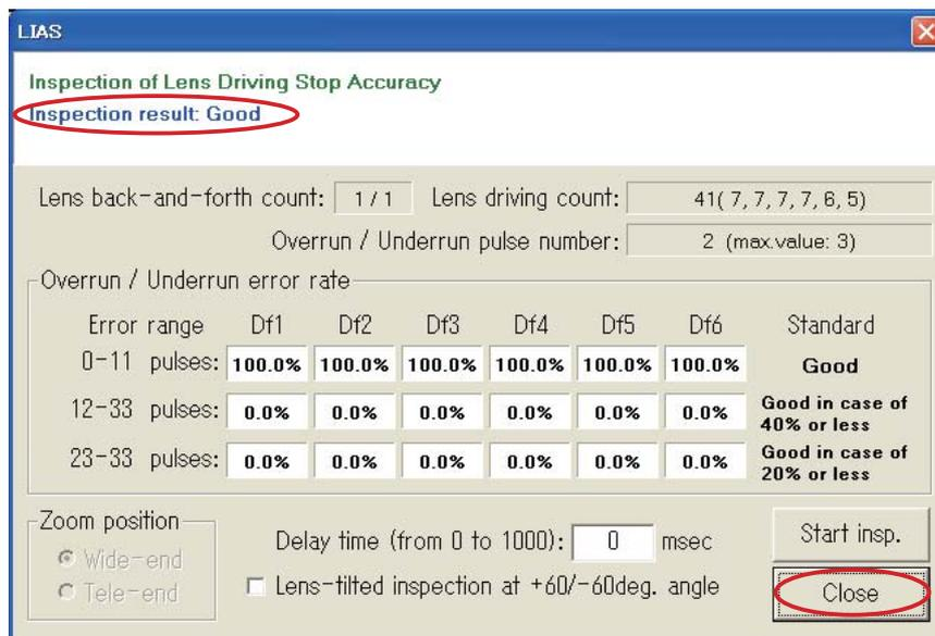
The number of overrun/underrun pulses must be within the following standards after the lens back-and-forth driving 1-motion.
