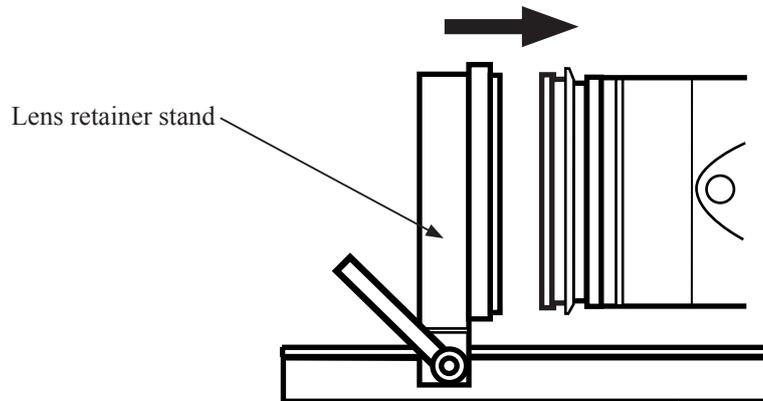
2. When the lens retainer stand is positioned as shown below, fix it by tightening the clamp.
