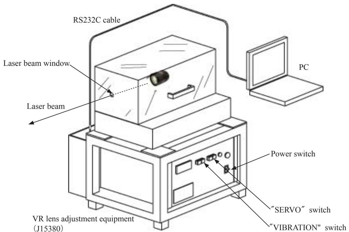
**Notes:** Keep the approx. 5-m distance from the laser beam window to the radiated surface.
