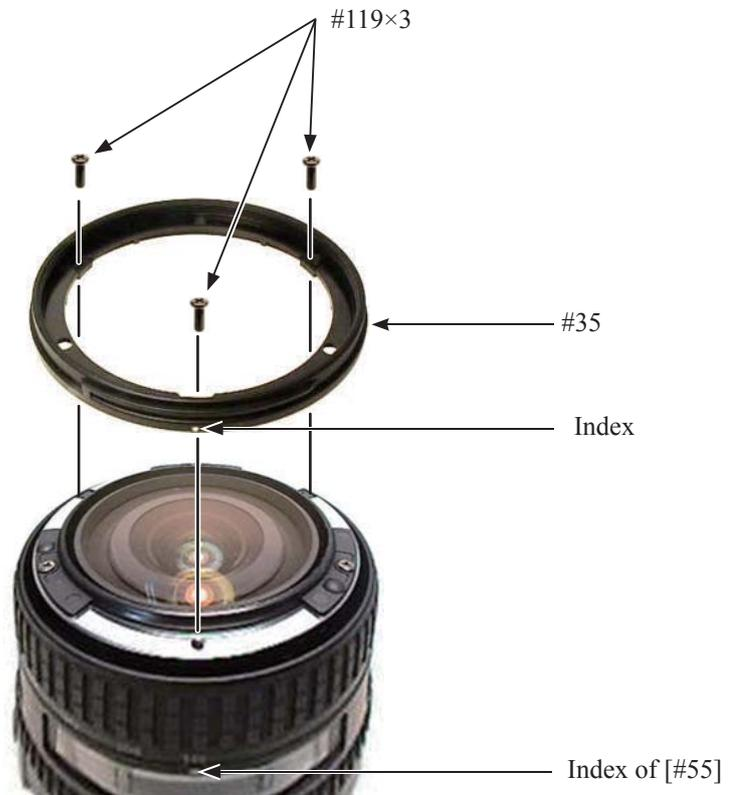
Adjustment of Focus movement (T, W)
