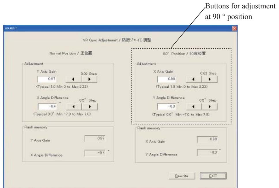
11. After the adjustment, click "Rewrite" button to write the adjustment value in FLASH-ROM of the lens.
