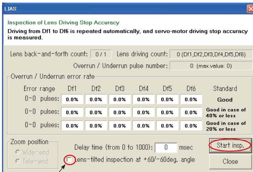
Tick here when measuring with the front lens group facing 60° angle up/downward.
