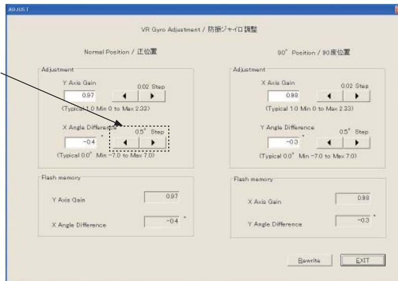
7. Adjust the vibration width by the buttons for Gyro-gain adjustment so that the measured vibration width at the center ( $\alpha'$ ) of the laser beam becomes 1/8 or less of the maximum width.
