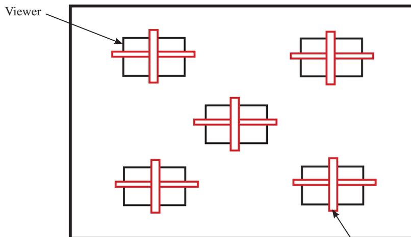
To prevent viewers falling off, attach Velcro tape on the back of the cardboard. Here in this document, 2mm-width tape is used.
