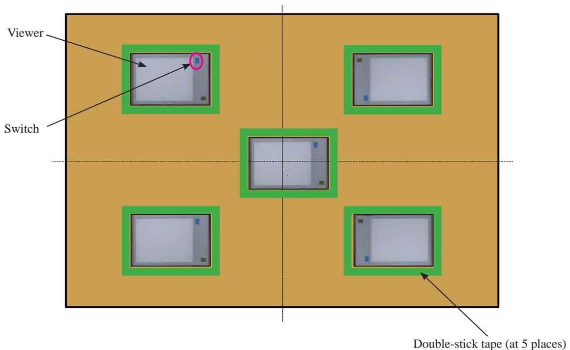
⑥ Light up the viewers. Set and attach the alignment chart (J19134) so that all the pinholes are located on the viewer.
