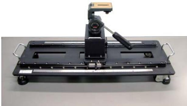
Slide rail for lens alignment equipment
